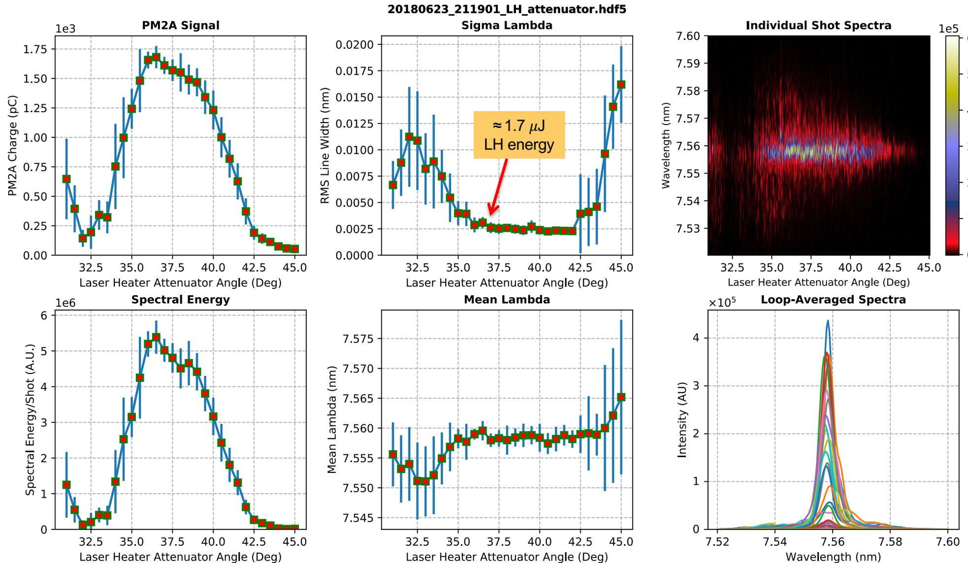
Note that FEL power is optimized at LH energy of  $\sim 1\text{-}2 \mu\text{J}$
