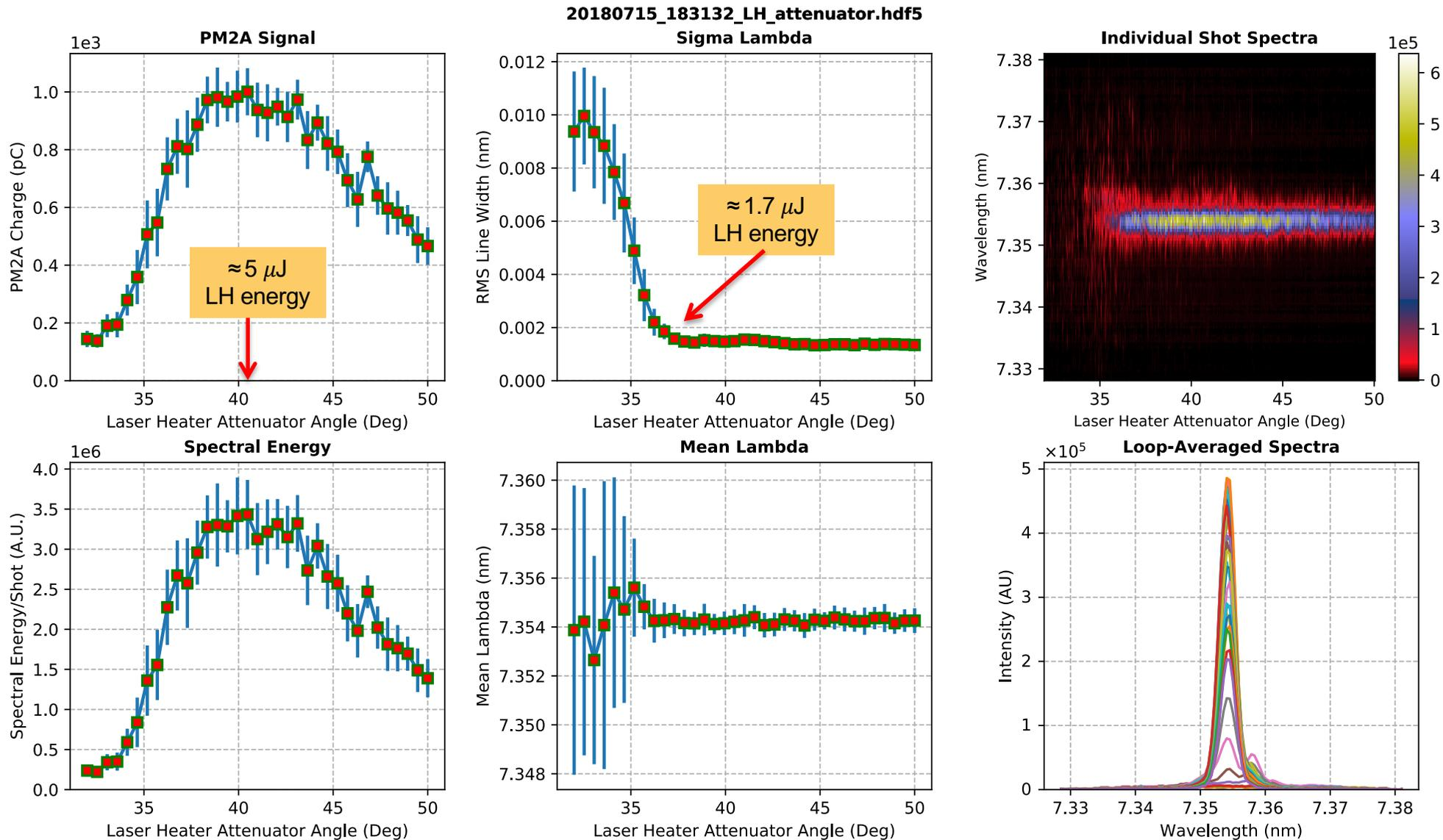
Note that FEL power insensitive over LH energy range of  $\sim 2$  to  $8 \mu\text{J}$  --- very different behavior than HGHG result
