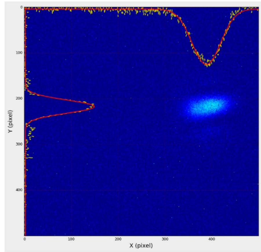
The transverse laser beam size is about 1mm, which is much larger than the electron beam
