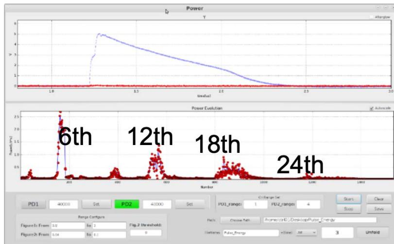
Scan the Gap of U40 and get coherent signal at various harmonics
