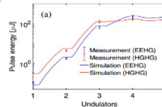
Lasing of the 1<sup>st</sup> stage HGHG at 6<sup>th</sup> harmonic and get coherent signal from the 2<sup>nd</sup> stage HGHG with "fresh bunch"
