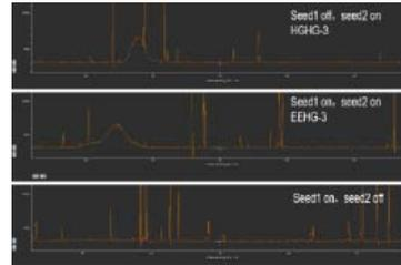
Amplification of the 1<sup>st</sup> stage EEHG. Pulse energy of the 3<sup>rd</sup> harmonic radiation exceeds 1 mJ
