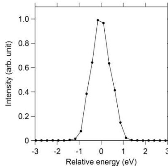
Averaged spectrum of the seed measured with a Si(220) channel-cut crystal. The number of accumulation at each point is 100 shots. The central photon energy is 10 keV
