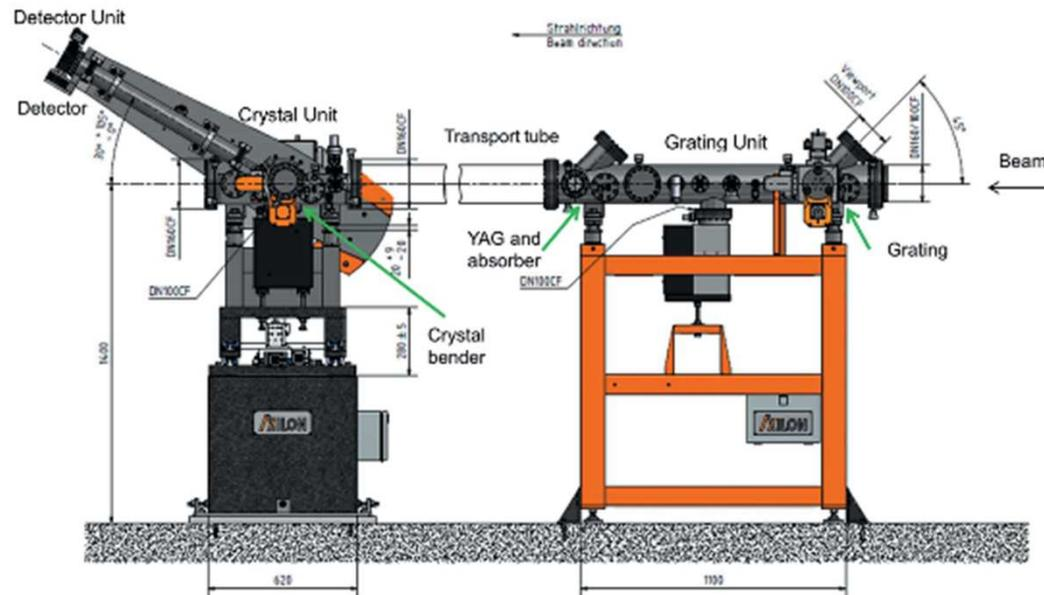
HIREX spectrometer at SASE1 from J. Gruenert et al, JSR 26, 1422 (2019)
