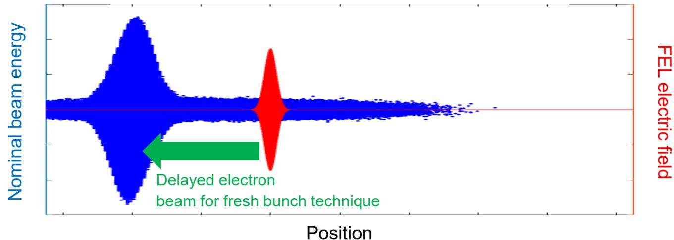
Schematic drawing of phase space after electron delay
