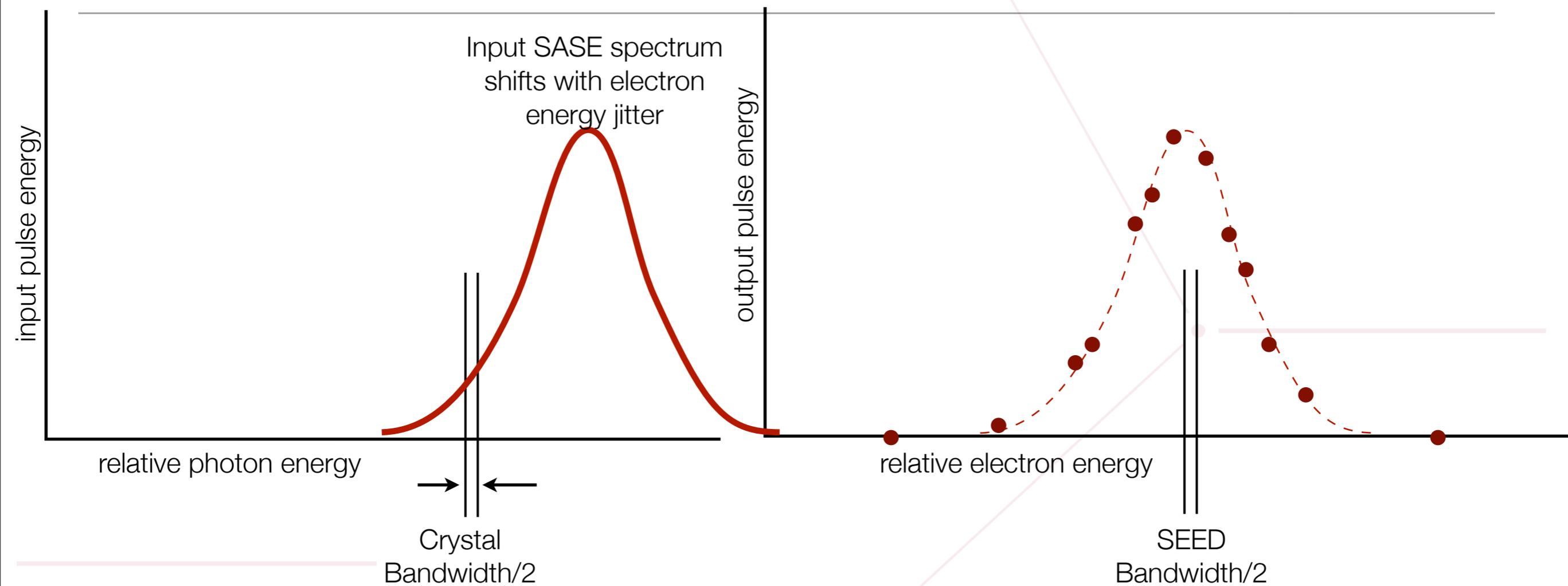
Jitter induced seeding power fluctuations depend on the ratio of jitter to input SASE bandwidth.
