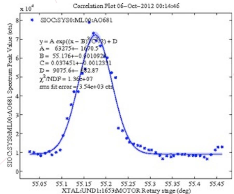
**3.** Fine tune crystal angle to maximize peak spectral density
