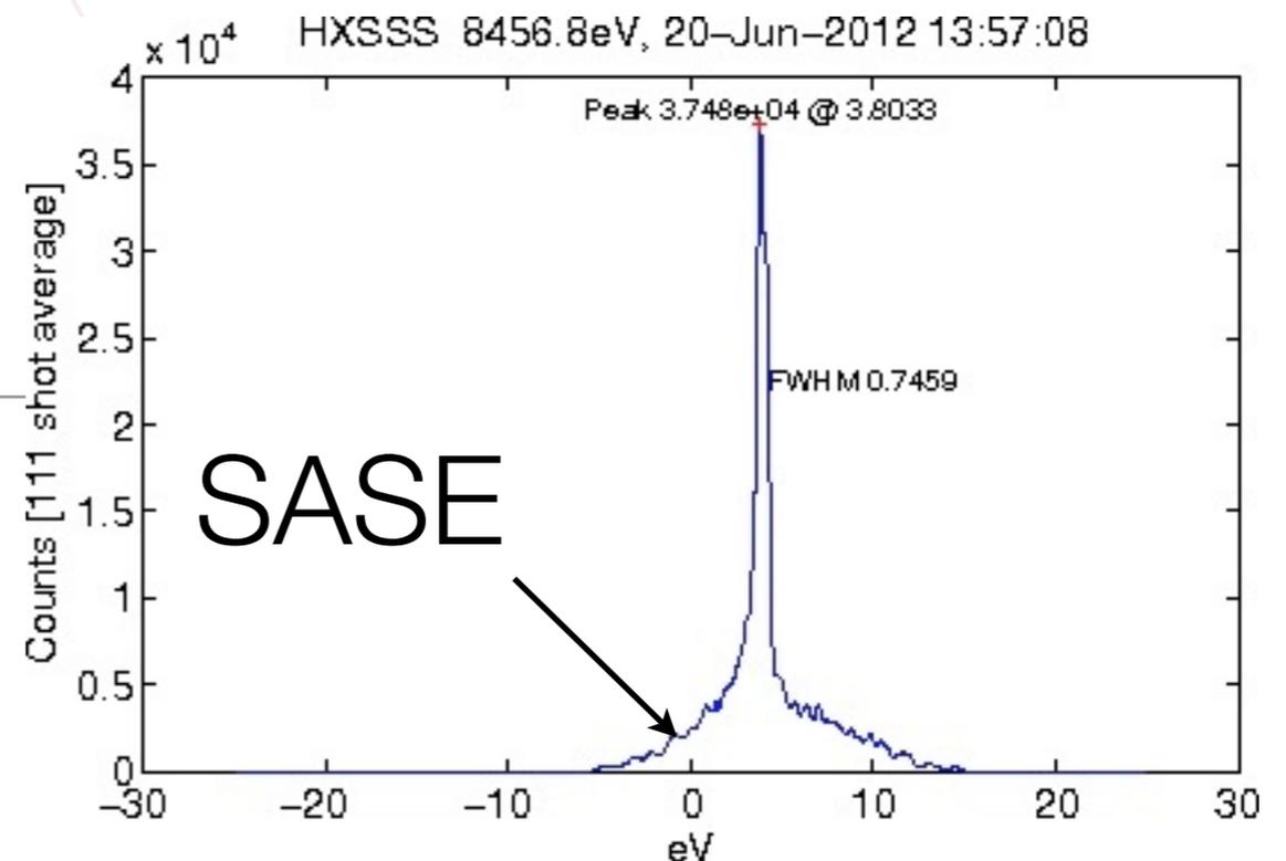
Not well-tuned beam showing substantial energy in SASE bandwidth.
