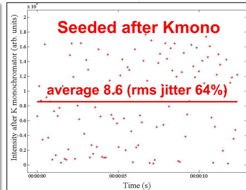
Adjusting for the additional attenuation of the seeded beam ( $8.6/0.7=12.3$ ), its intensity is **3.4 x SASE**.
