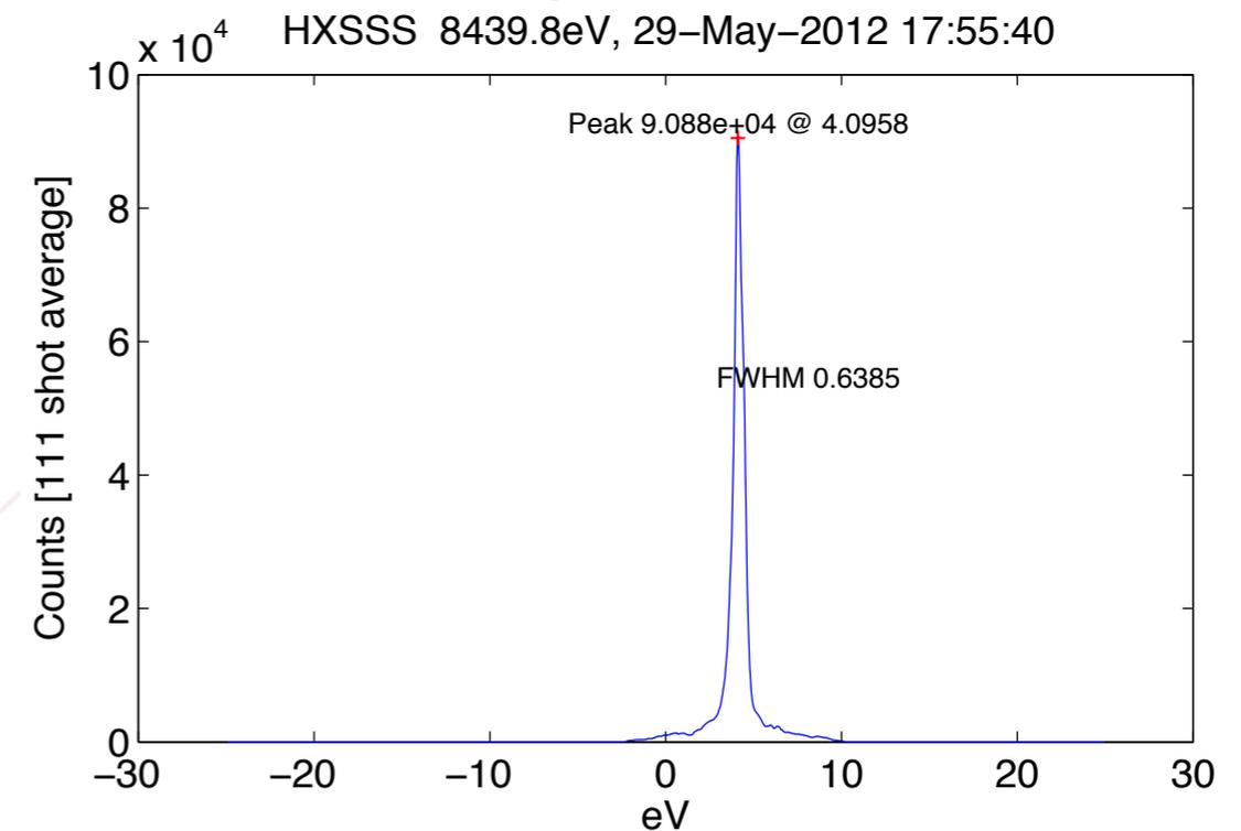
Well-tuned beam. Most energy is in the narrow peak.
