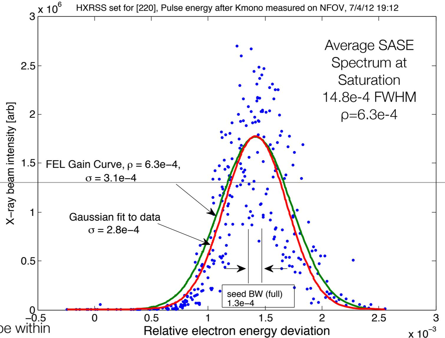
Theoretical SASE spectrum at saturation point follows  $\exp(-0.5 \cdot (e_{\text{photon}}/\rho)^2)$ ; expressed in relative electron energy deviation, is half as broad.
