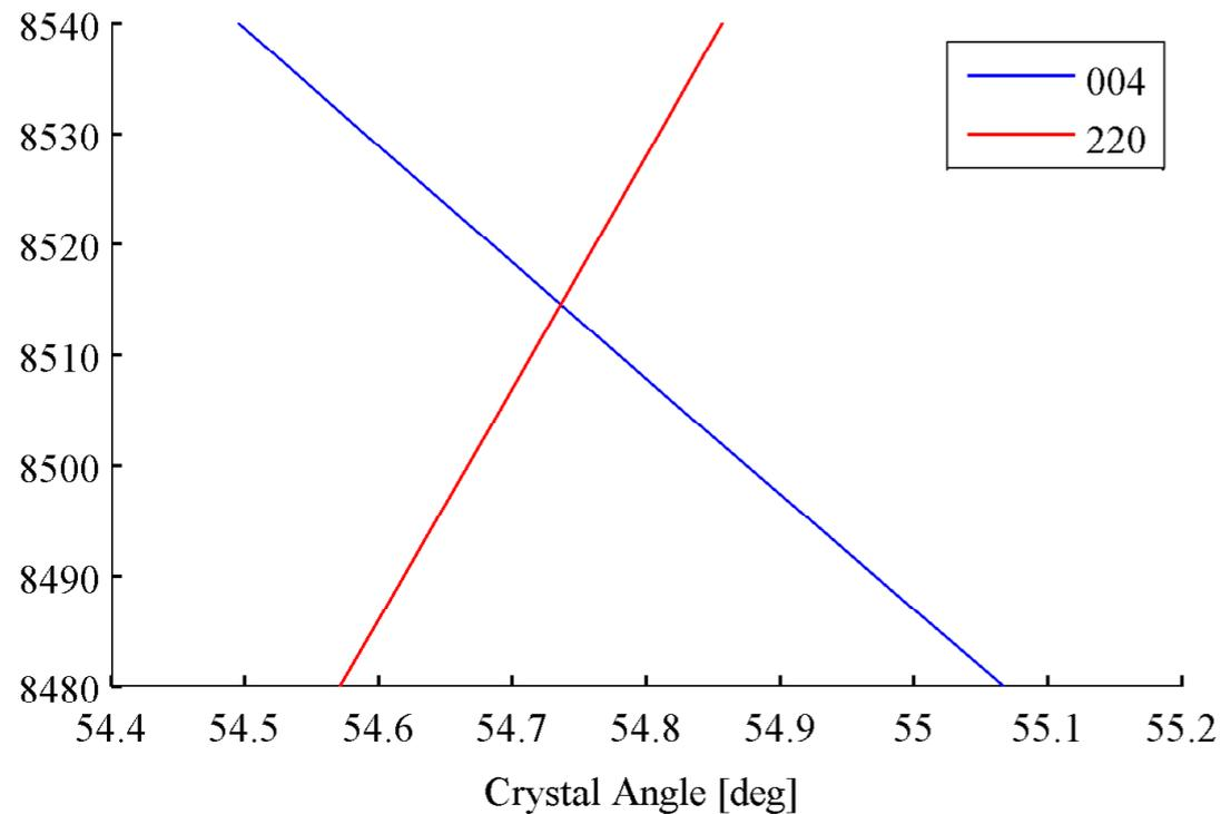
Photon energy versus crystal angle for 004 (Bragg) and 220 (Laue) reflection
