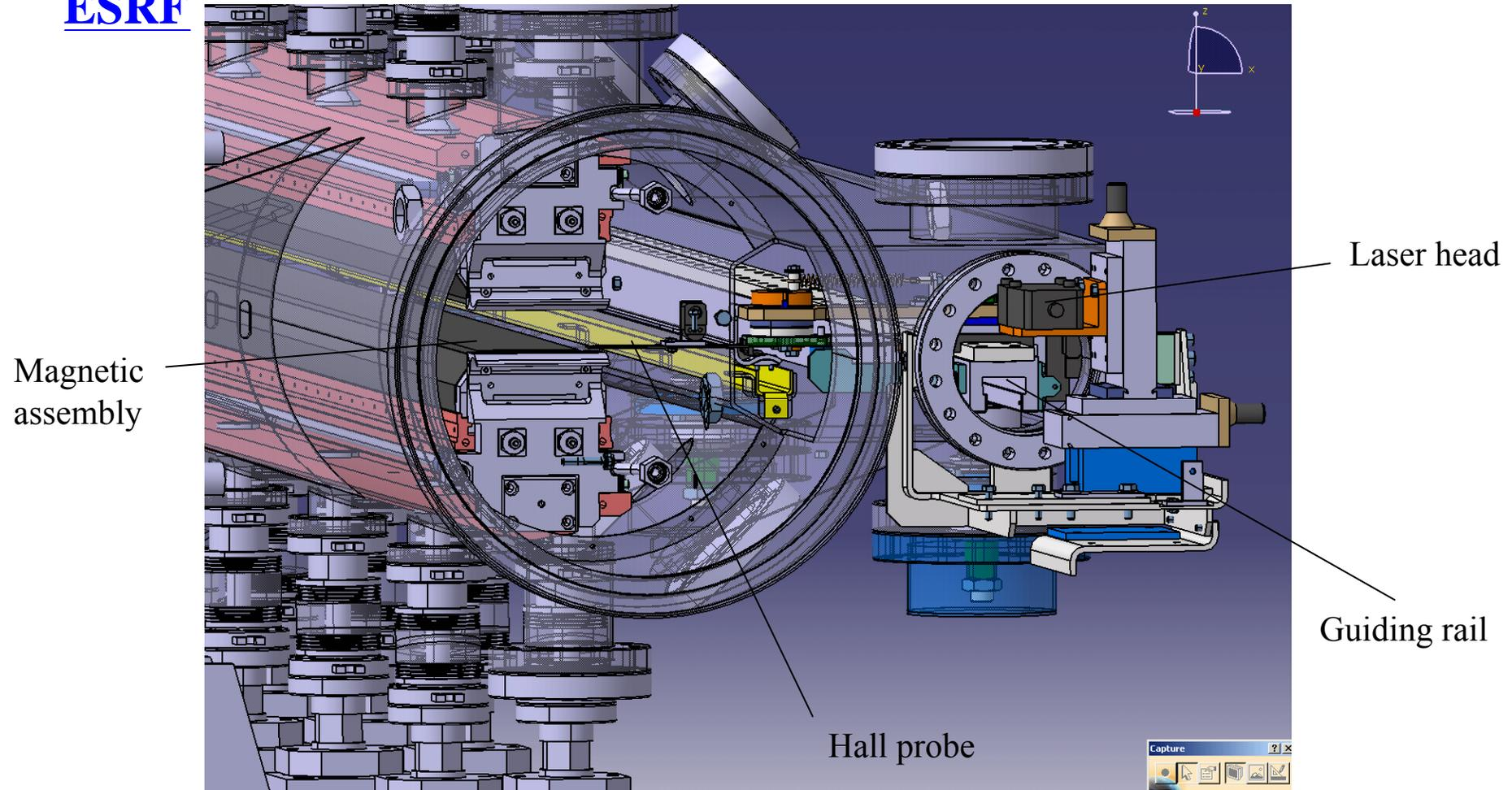
Longitudinal motion: magnetically coupled with an external axe (old hall probe bench) -> fast scans
