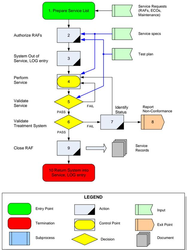
Figure 3. Work flow for completing a Repair/Action on the Proton Therapy System.
