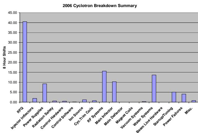
Figure 4. Cyclotron System breakdown summary for 2006. Improving RFQ reliability is a high priority.
