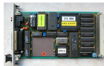
Fig. 7: TMS 9995  $\mu$ C board (above)
