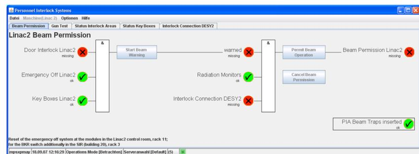
Fig. 1: Screen shot of beam permission operation program
