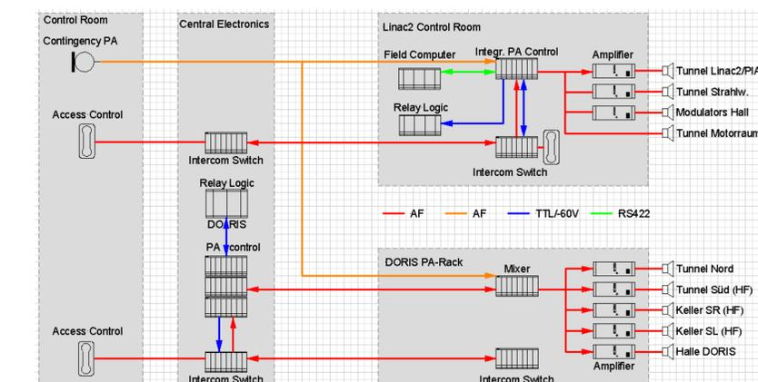
Fig. 2: PA system signal flow diagram (simplified)
