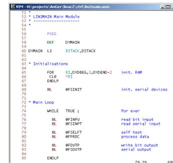
Fig. 8: Main loop of the program (right)
