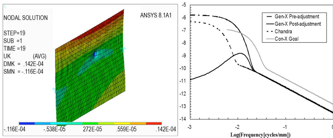
**Figure 2. (Left) A finite-element analysis of the influence function for a piezoelectric bimorph zone on a thin mirror; (Right) schematic illustration of the suppression of low-frequency figure errors to correct a mounted mirror to meet the Gen-X requirements on imaging quality.**
