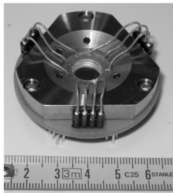
Fig 1: Prototype of bidirectional actuated membrane mirror.
