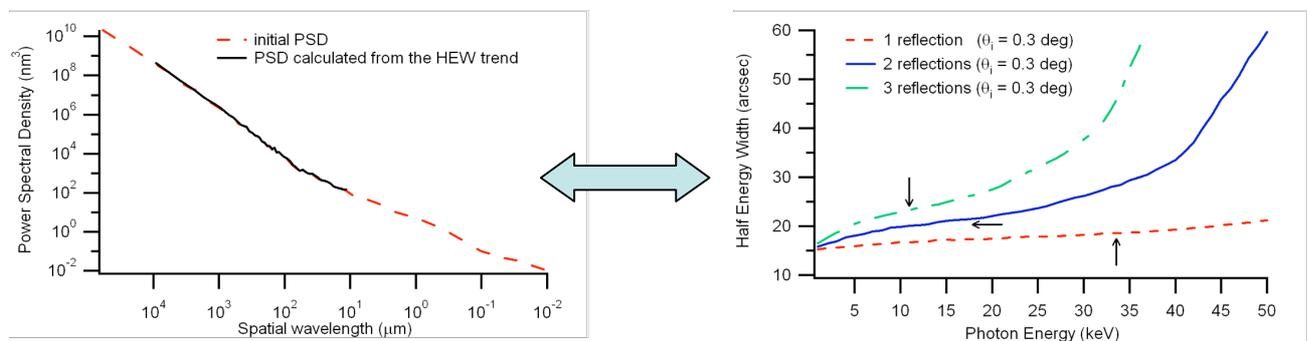
Fig. 1: an example of computation of the HEW scattering term (right panel) from the PSD (left, dashed line) of the surface of an hypothetical X-ray optical system with 1,2,3 reflections at the same grazing incidence angle of 0.3 deg, and vice versa.
