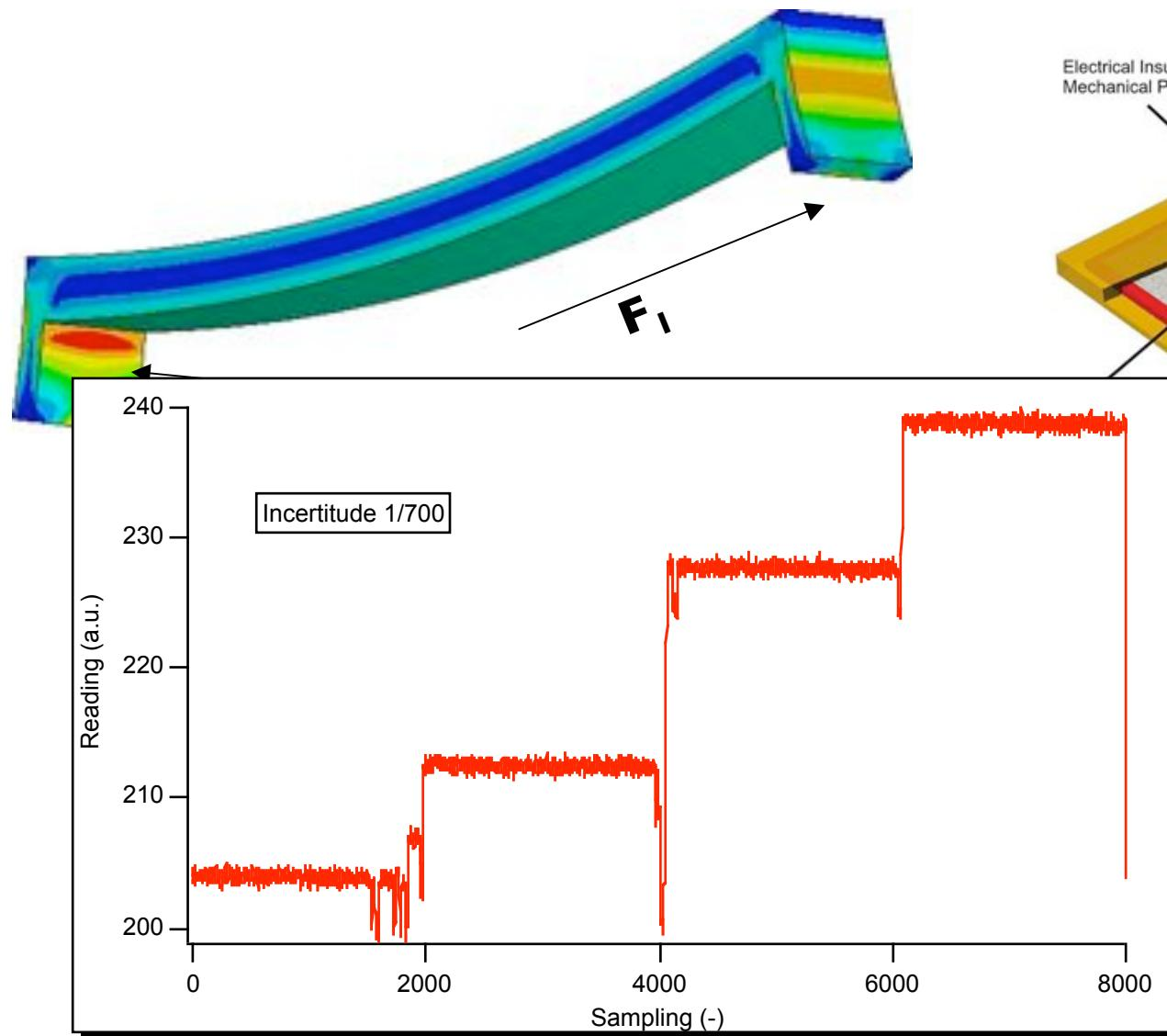
Measurement of the local radius of curvature using strain gauges glued on the back of the mirror
