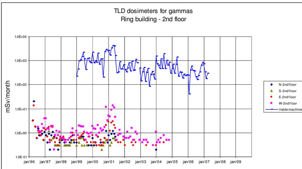
Fig.6 - Monthly doses from TLD dosimeters placed at N, S, E and W sides, in the 2<sup>nd</sup> floor of the ring building.
