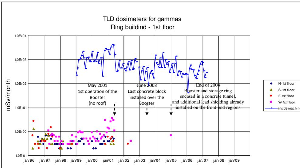
Fig.5 - Monthly doses from TLD dosimeters placed at N, S, E and W sides, in the 1<sup>st</sup> floor of the ring building.
