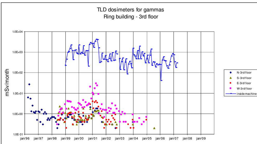
Fig.7 - Monthly doses from TLD dosimeters placed at N, S, E and W sides, in the 3<sup>rd</sup> floor of the ring building.
