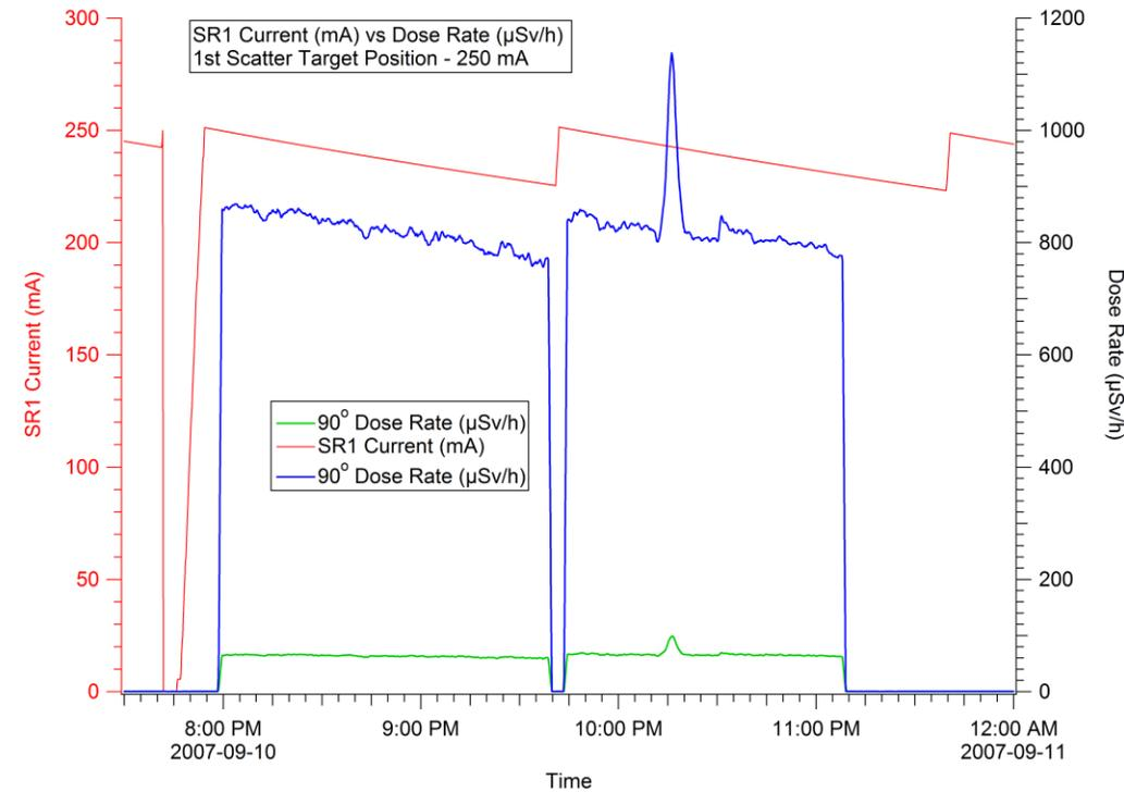
NOTE: The spike in the radiation levels seen on both radiation monitors was due to an adjustment that was made at another insertion device magnet. The adjustment caused a perturbation in the electron beam orbit, which resulted in the observed increase in the radiation levels measured near the scattering target. When the beam orbit was returned to normal, the radiation measured returned to the previous levels.
