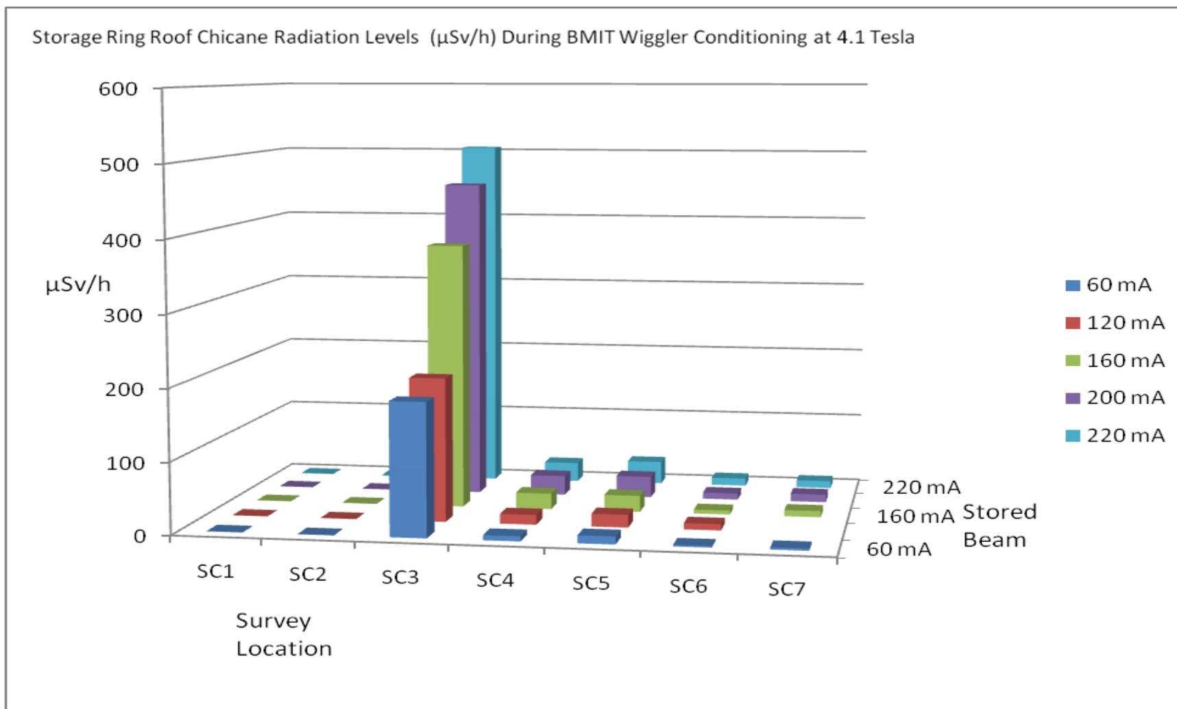
**Storage Ring Roof Chicane Radiation Levels During BMIT Wiggler Conditioning on February 19, 2008**
