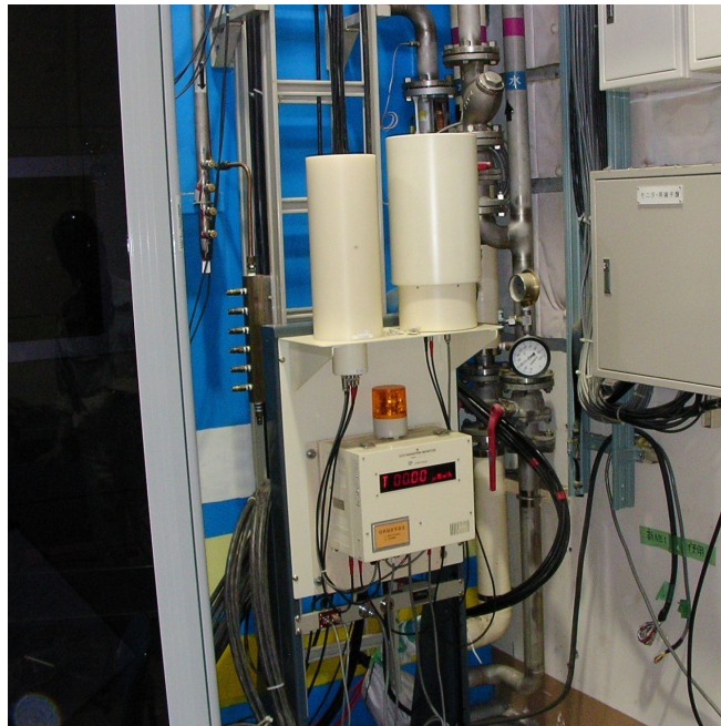
Fig.3 - An ORG monitor consists of a 10-liter ionization chamber for gamma detection and a 1-inch BF3 proportional counter for neutron detection.
