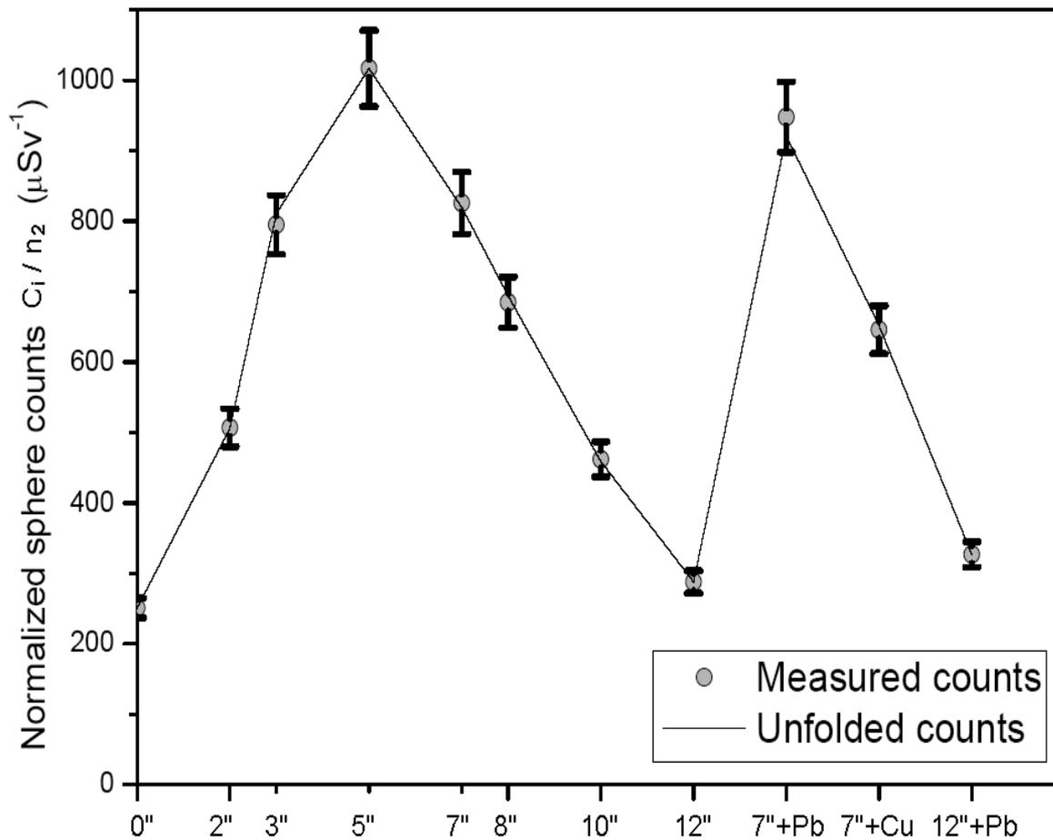
The “unfolded counts” are calculated by applying the response function of each sphere to the spectrum unfolded with FRUIT.
