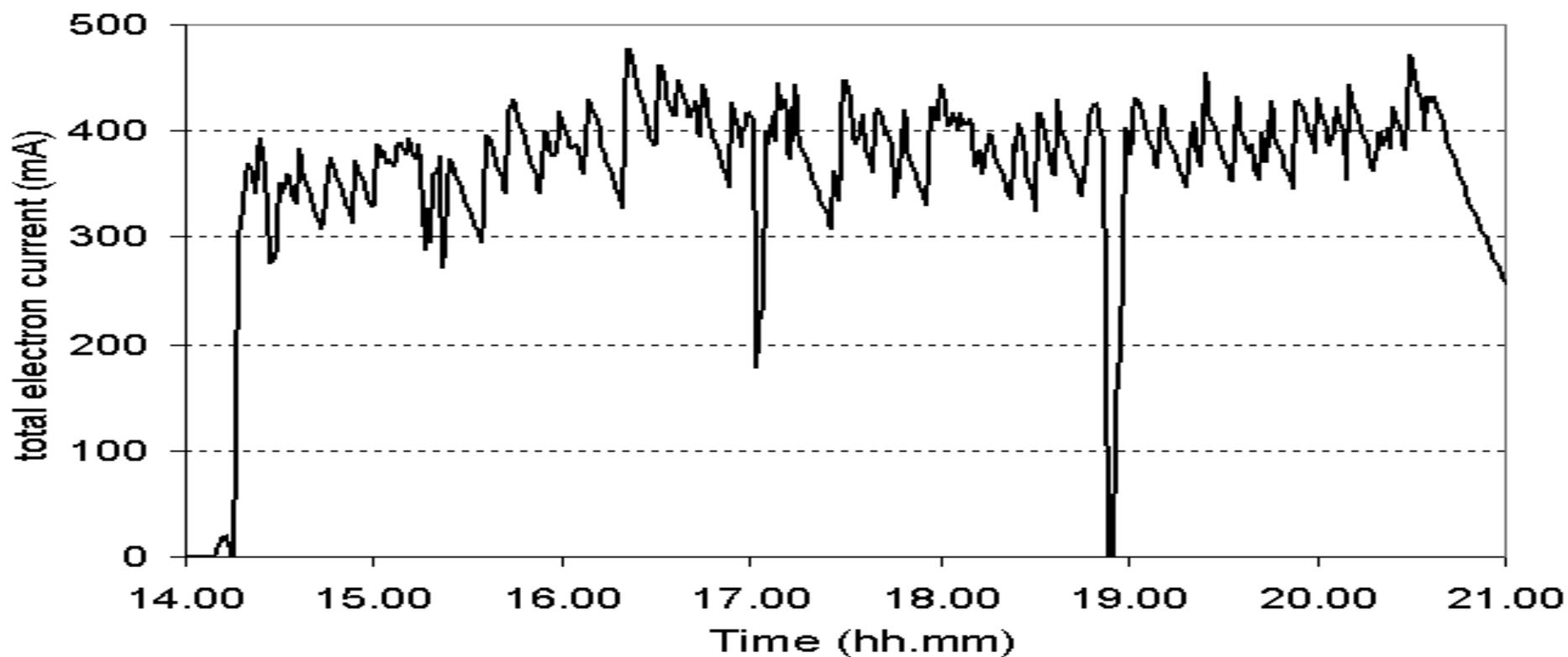
The radiation leakage from DAΦNE depends in a complex way from the injection parameter, the stored current, its temporal variability and a series of non predictable events such as the beam losses.
