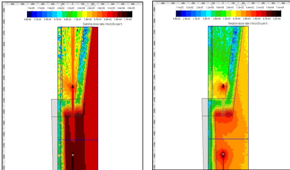
Fig.3 - Gamma and neutron dose rates from grazing incidence beam loss at insertion device.
