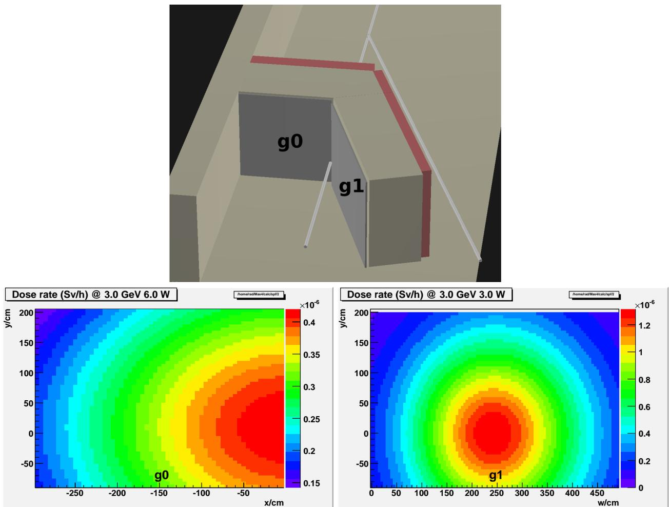
Table 6 – The calculated dose rates for the SPF. Top: the SPF layout showing the two grids on which the dose rates were calculated. Bottom: the dose rate on the the forward (g0) and side (g1) grid.
