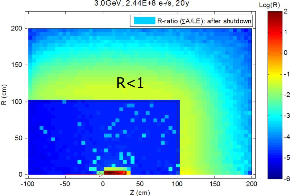
Residual Activity Zoning for the Concrete Silo with a Fe Target
