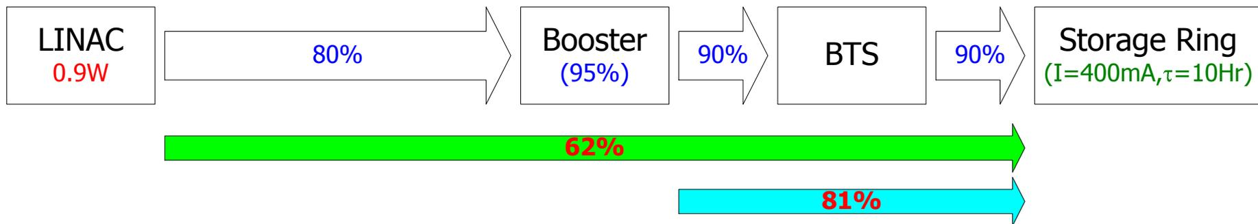
**TPS Operation:** Extraction/Transfer/Ramping/Injection Efficiency
