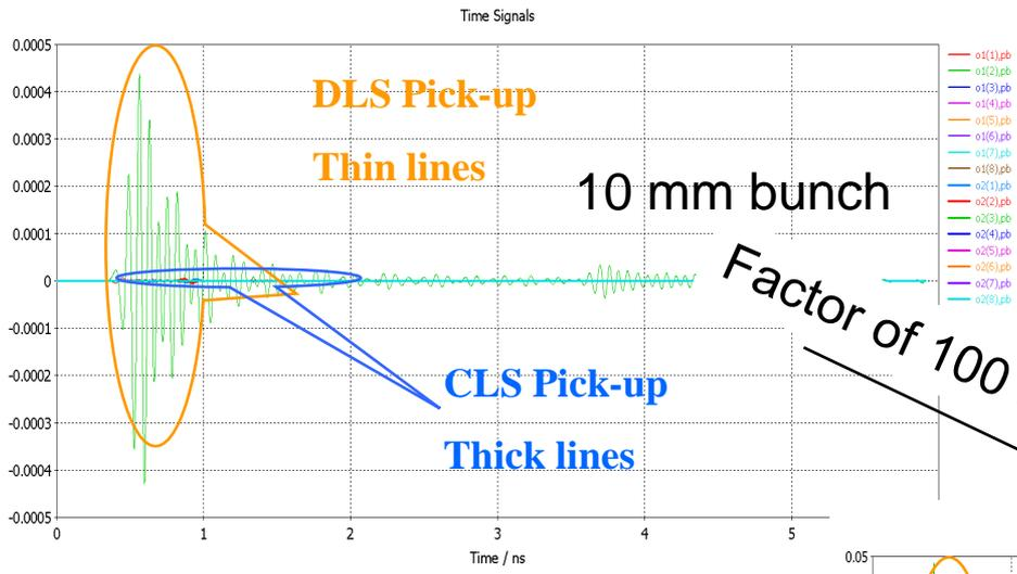
The EM signal induced by the beam propagates in many modes through the pick-ups.
