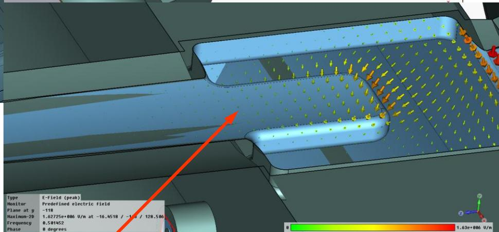
TM010 E field from Eigen mode solver near coupling tongue
