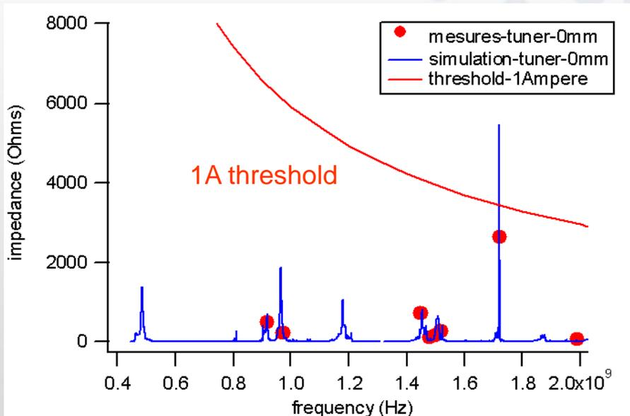
All the **longitudinal HOM impedances** are well below the threshold of 1A / 18 cavities
