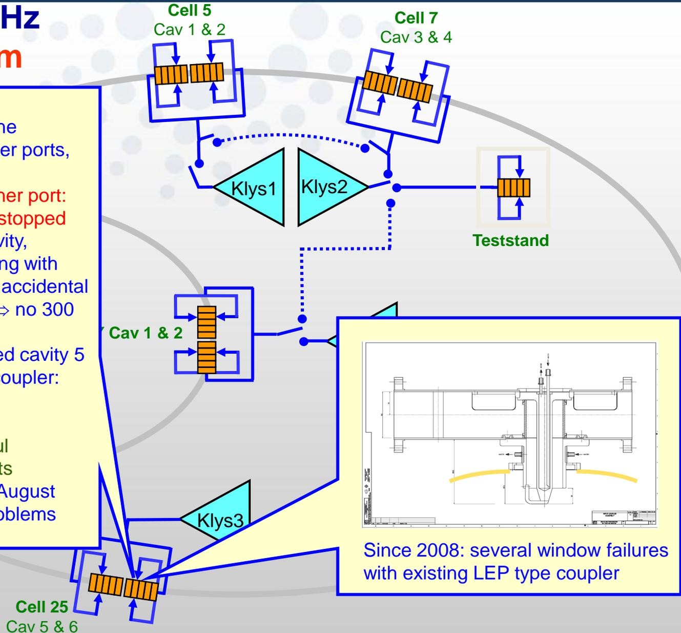
Since 2008: several window failures with existing LEP type coupler
