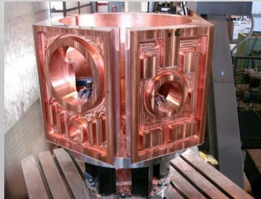
*CINEL: 3 body sectors after machining of the water cooling channels, September 2010*
