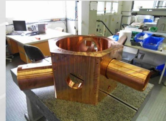
*RI: Body after e-beam welding of the HOM coupling sections, April 2010*
