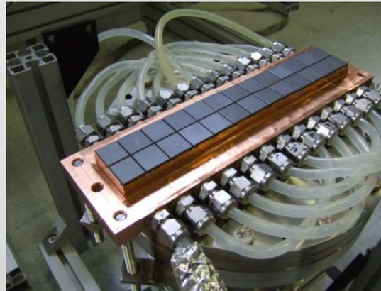
*RI: Ferrite HOM absorber for IR thermal test at ESRF, April 2010*
