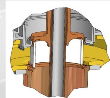
LHC window directly brazed into copper collars:
