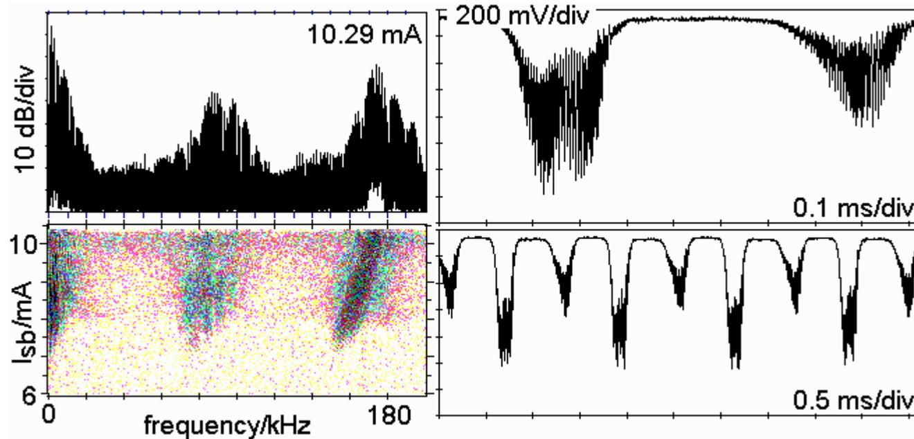
single bunch CSR signal observed between 100 GHz and 1 THz
