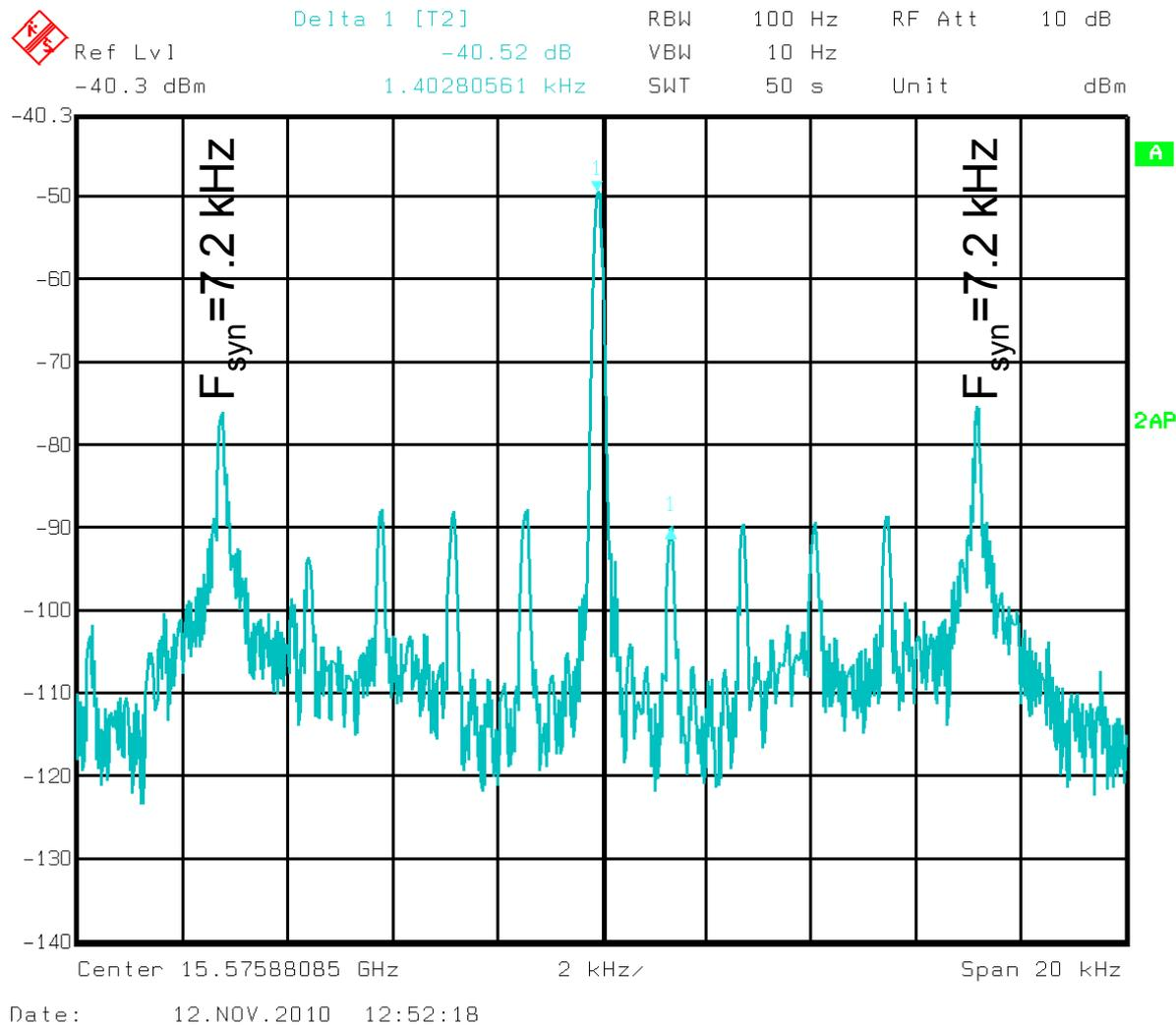
**Pick-up signal of a single bunch with 8 mA observed at 15.6 GHz**
