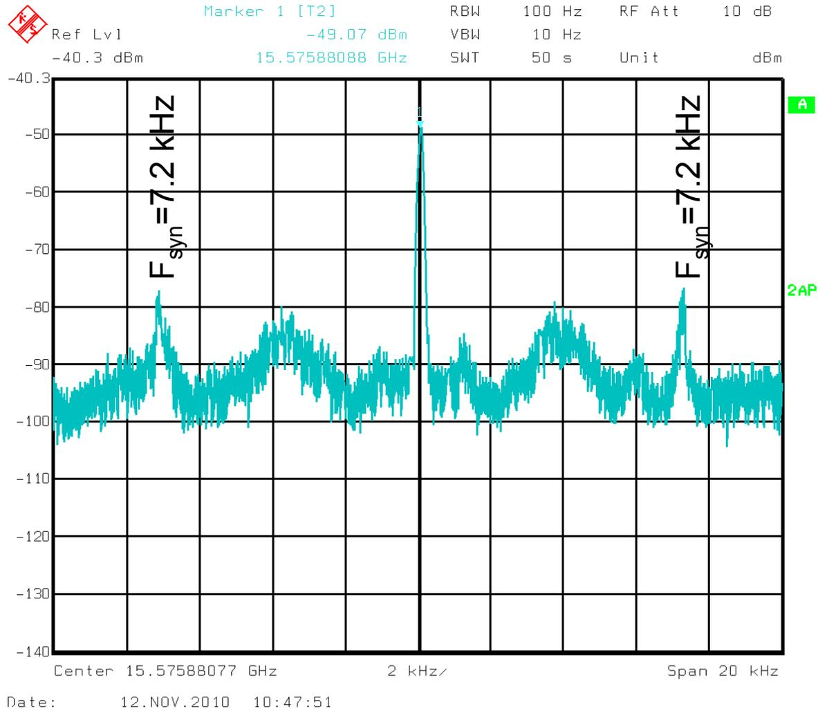
**Pick-up signal of a single bunch with 15.7 mA observed at 15.6 GHz**
