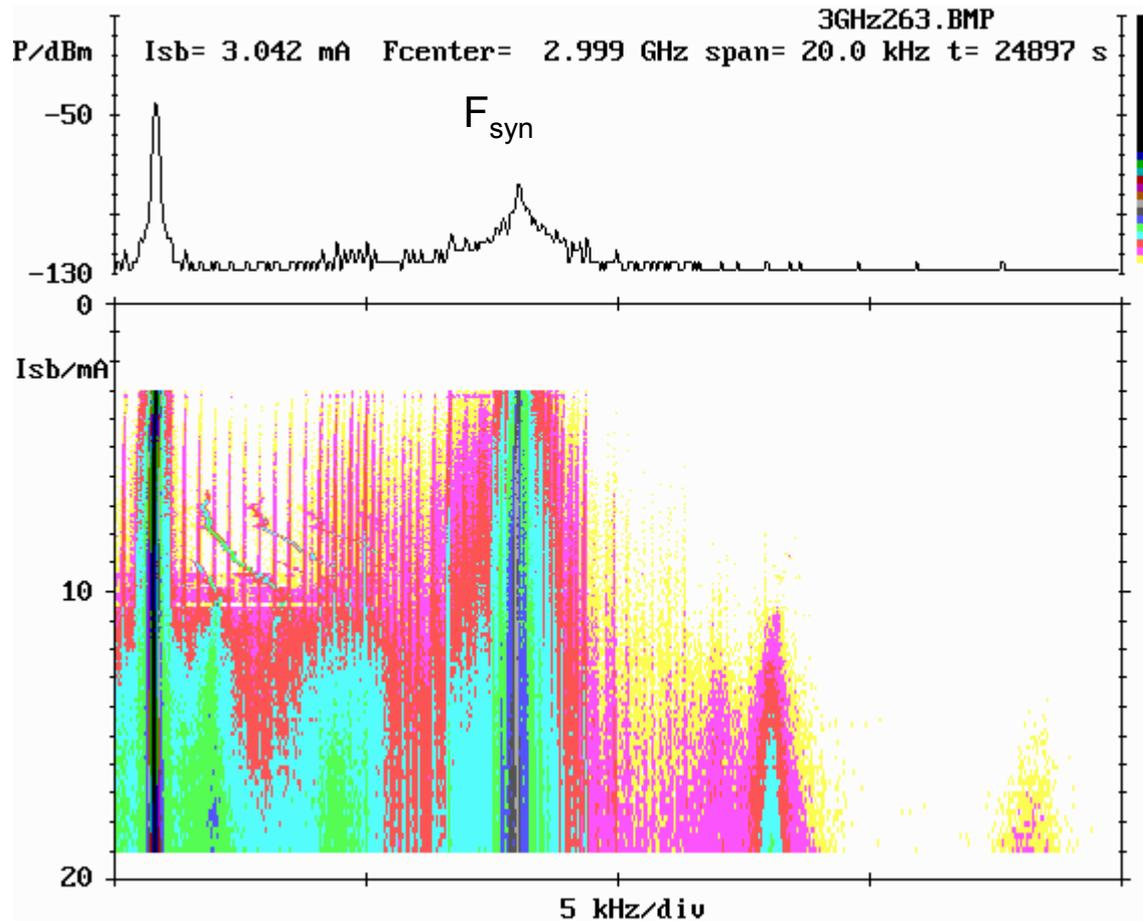
**stripline signal of a single bunch observed at 3 GHz**
