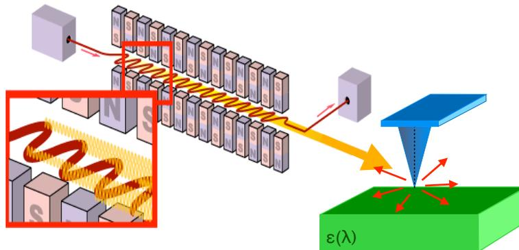
Fig. 1: SNIM setup in combination with the free-electron laser FELBE.
