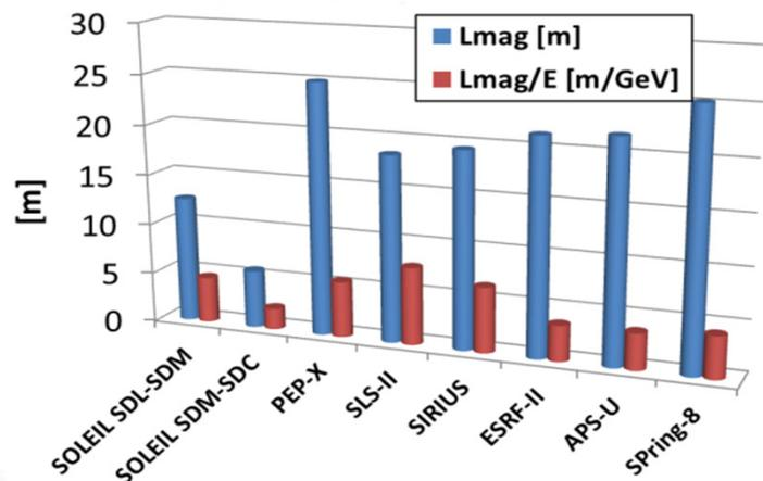
The lengths dedicated to magnets are relatively short; 12.5 m in SDL-SDM and  $2 \times 5.73$  m in SDM-SDC-SDM.
