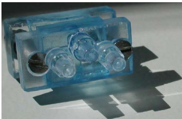
**Figure 1.** Mechanically fabricated mixer with cross channel. Triangle cross section 100 $\mu\text{m}$  high, 200 $\mu\text{m}$  wide.
